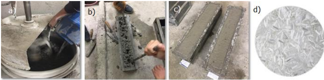
Figure 1. Production of the Test Specimens: a) Concrete mixture, b) rodding, c) molded concrete, d) micro synthetic fibers added into the concrete mixture
