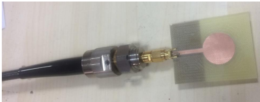
Figure 8. Fabricated planar circular shaped monopole antenna
