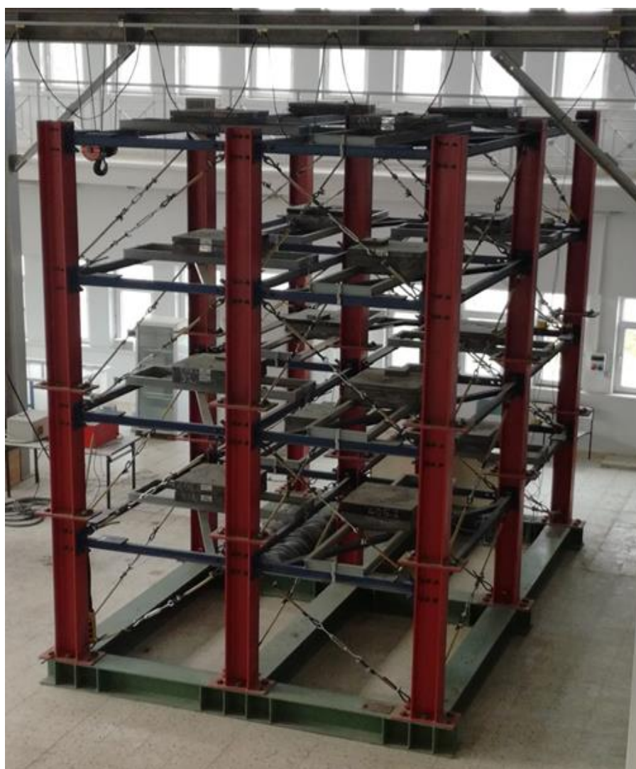
Figure 1. Formation of steel test structure reinforced with cable element
