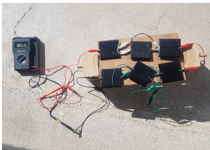
Figure 2. Photo of the constructed system consisting of 6 solar cells on the platform together with a multimeter during the experiments.
