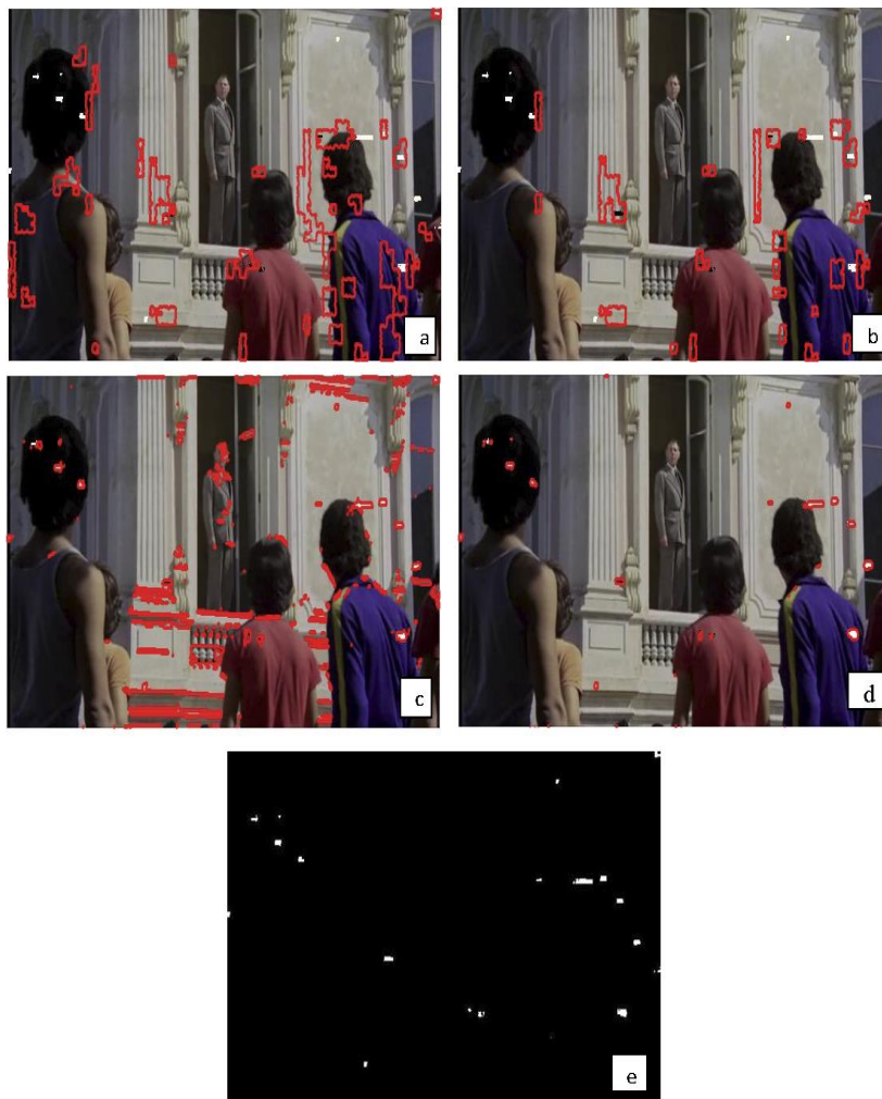
Figure 3. Results of different colored artificial blotch detection studies for "hababam" moving image sequence: a) HOG feature, b) LBP feature, c) SROD, d) Proposed method and e) Mask image showing blotched areas.
