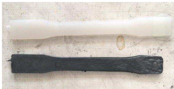
Figure 1. Prepared samples the white is MDPE-HA and the black is MDPE-HA-SiC.
