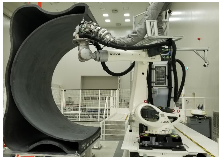
Figure 2. Example of tool; Composite fiber placement tool
