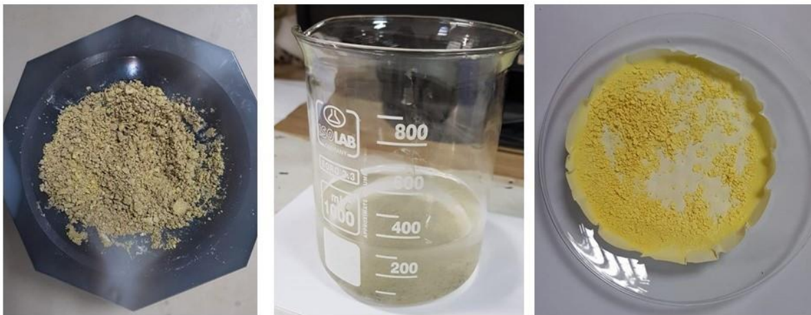
Figure 1. The visual summary of SPRT synthesis method. Co-grinding of species, suspending of ceramic powders in water, centrifugation and drying of the powders
